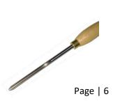
Tips: Begin with the tool handle low and rub the heel of the bevel against the wood. Slowly raise the handle until fine shavings appear then rotate and angle the tool slightly in the direction of travel. Always cut downhill (from the highest point to the lowest point).
