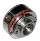
Scroll chucks with a solid back plate will require much less maintenance as the gears are protected from dirt and dust. A chuck with jaws that are capable of gripping internally and externally is recommended as this greatly reduces the number of jaw sets required.
