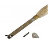
Vases, hollow forms and undercut rims on bowls can easily and safely be produced using a hollowing tool. For small to medium sized projects a hollowing tool with swivelling scraper tips is ideal. Scraper tips are easy to sharpen and can be replaced if needed. For larger pieces a deep hollowing tool should be used with a cutter system that slices through the wood rather than scraping it.
