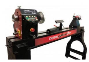
A powerful motor suitable for extended periods of use is ideal. Lathes with electronic variable speed will save the time and frustration of having to move the belt along pulleys to achieve the correct spindle speed. Slower speeds need to be used for roughing and initial shaping, higher speeds need to be used for finishing — a variable speed unit allows the speed to be changed instantly while the lathe is running.
